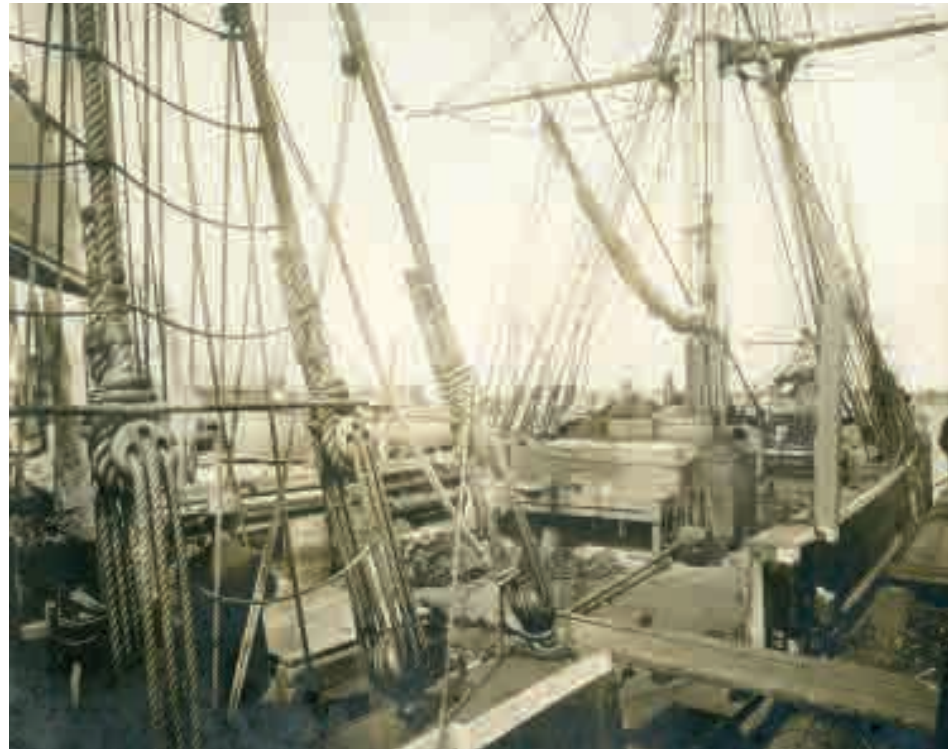
Above: Detail of the main starboard standing rigging of the bark Kathleen at wharfside, New Bedford, circa 1900. Left: Clifford W. Ashley, The Ashley Book of Knots. Doubleday, Doran, & Company, Inc.: Garden City, New York, 1944. Page 254.
