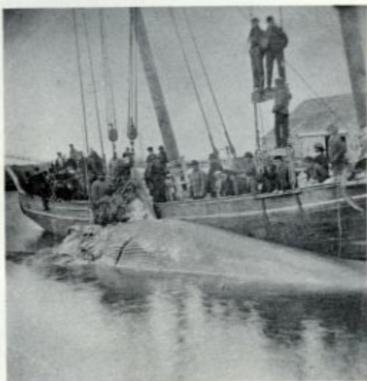
Unidentified schooner, date unknown, cutting in a finback whale. The left view shows cutting staging in its pre-1860 form
