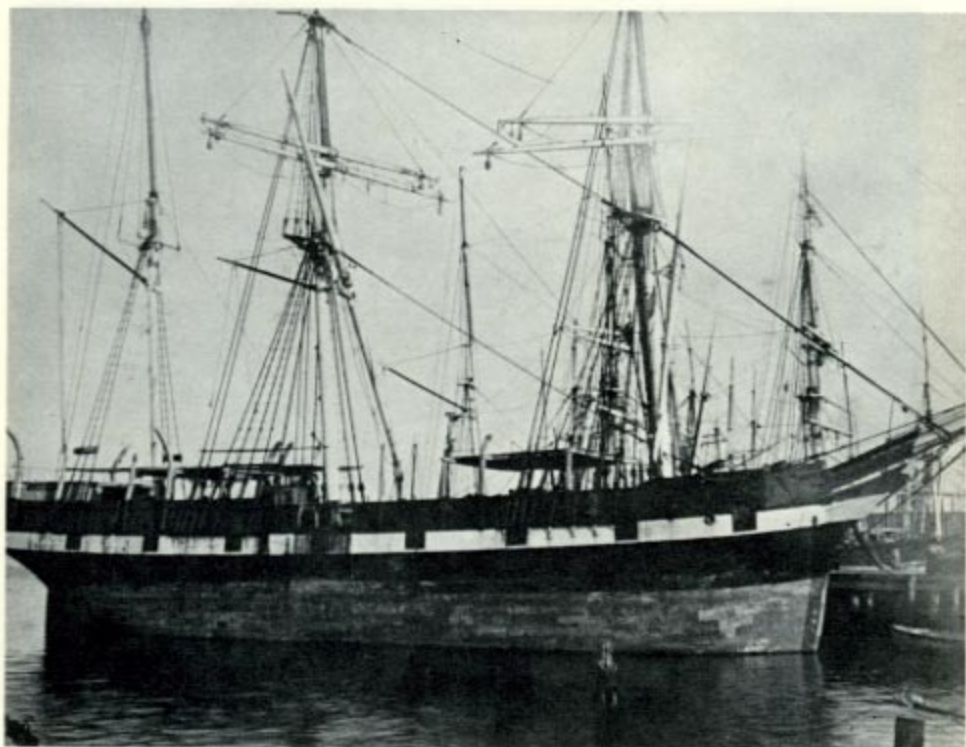
Bark, ex-ship, Lagoda , 340 62/95 tons (371.15 tons, new register). Built at Scituate, Mass., 1826; converted to a whaler and reregistered at New Bedford, 1841; converted to bark, 1860; based at San Francisco, 1888-1889; condemned at Yokohama and sold, 1890
