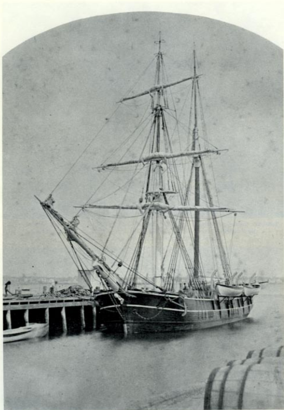
Brig Abbott Lawrence , 159.81 tons. Built at Duxbury, Mass., 1849; reregistered at Fairhaven, Mass., 1867, as a whaler; reregistered at New Bedford, 1875; condemned and sold foreign, 1881. The term 'brig' was used loosely by whalers; most 'brigs' were probably hermaphrodites, particularly after 1840
