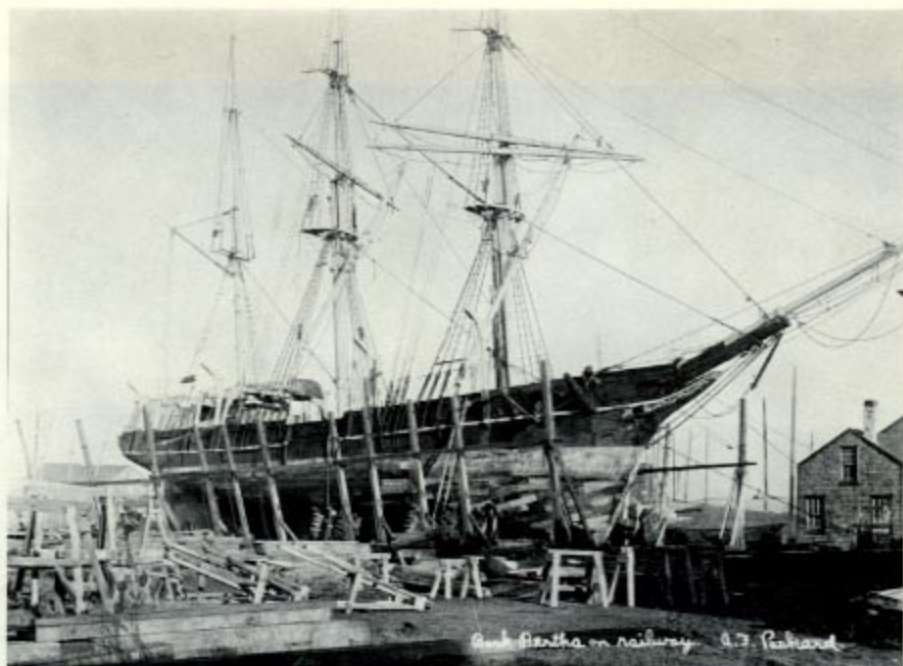
Bark Bertha , 177.37 tons, built at New Bedford, 1877, on the marine railway at Fairhaven. Date unknown
